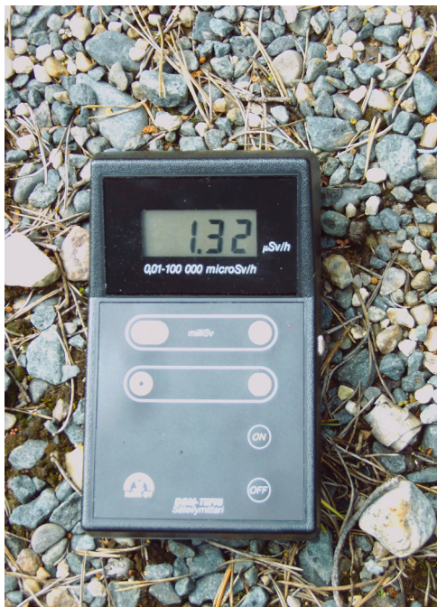
Figure 6. Radioactivity measured at the former gate, 1.32 \mu\text{S}/\text{h} . Photo: Alfred Colpaert 18.8.2004.
