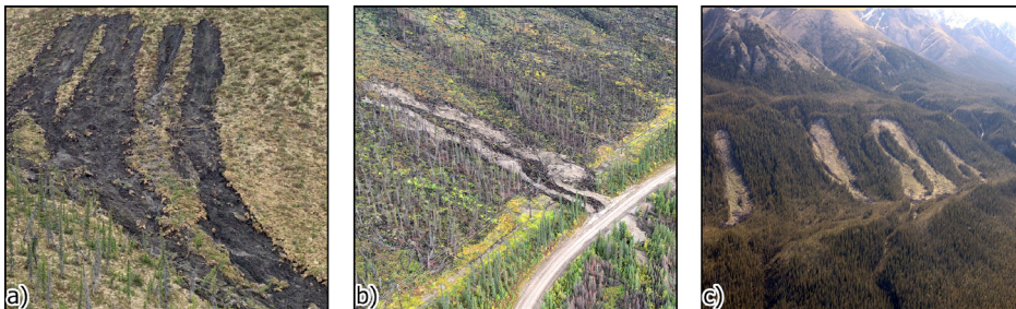
Figure 4. Active-layer detachment failure (ALD) photo compilation. Panel a) recent ALDs on the right side of Dempster Highway in Yukon at km 180-185 (photo taken Jun. 2025); Panel b) ALD that occurred after a 2023 forest fire adjacent to Haggart Creek Road, north of Mayo, Yukon, Canada (photo taken Aug. 2024); Panel c) ALDs on the side walls of the Donjek River Valley, Kluane Ranges, Yukon, Canada (photo taken in Jun. 2025). Photos: a) Eirini Makopoulou; b) Yukon Geological Survey 2024; c) Alix Varnajot.
